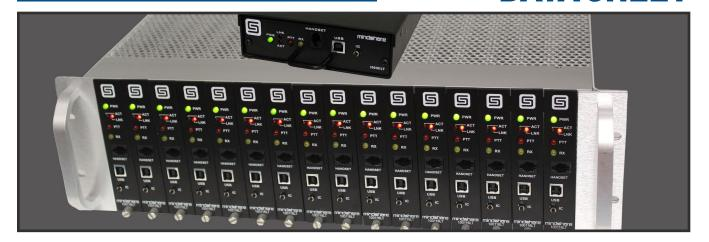
The Mindshare Radio Interface (MRI) is a Voice over IP (VoIP) endpoint device which acts as a console system gateway to control station radios and legacy analog interfaces. It is specifically engineered for radio control application and is designed to operate in the same environment as the radio equipment it interfaces with.
